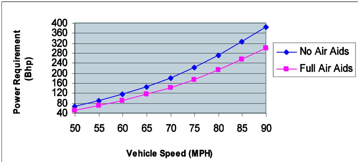
At approximately 0.3 lb./BhpHr fuel consumption, a reduction of 35 Bhp required to cruise at 65 mph results in a savings of about 10.5 lbs. of fuel every hour ( $0.3 \times 35 = 10.5$ ). Since diesel fuel weighs about 7.1 lb./gal., this amounts to a savings of 1.5 gallons of fuel saved every hour ( $10.5/7.1 = 1.5$ ). For a truck running 10 hours per day, that's 15 gallons of fuel saved per day. At \$2.45 per gallon of fuel, the dollar savings is \$36.75 per truck per day.
