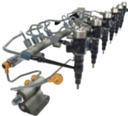
The ISX15 features our exclusive XPI fuel system. Of all North American manufacturers, only Cummins has the in-house capabilities to design and manufacture this critical element. The XPI fuel system is capable of the highest injection pressures in the industry, with a common-rail design that delivers strong performance independent of engine speed. Multiple injection events provide better fuel economy and help reduce engine noise.
