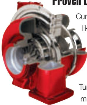
Cummins cooled-EGR subsystem isn't like the exhaust gas recirculation systems found on other diesel engines. It's simpler and more robust. Together with our patented Holset Variable Geometry Turbocharger (which has only one moving part in the hot exhaust stream for reliability and durability) it's a total
