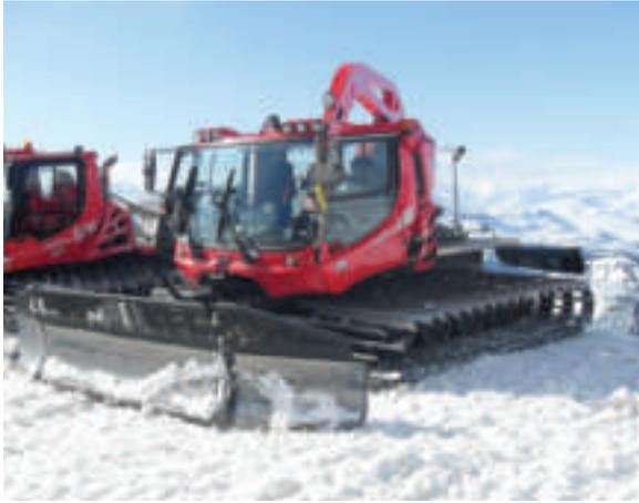
**Operating in the Alps, a snow groomer on a field test with a Tier 4 Interim/ Stage IIIB QSL9 engine performs more effectively at high altitude than the previous Tier 3/Stage IIIA engine.**
